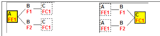
Figure 3: Failure nets: on the left focus on top failure, on the right focus on failure cause
