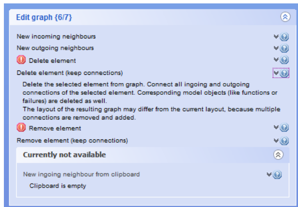
Figure: Graph Editor – available option with shown explanation / unavailable option with shown explanation
